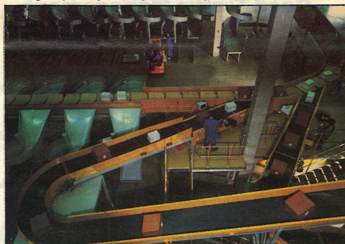
Goods are automatically sorted into customer pallet loads.
